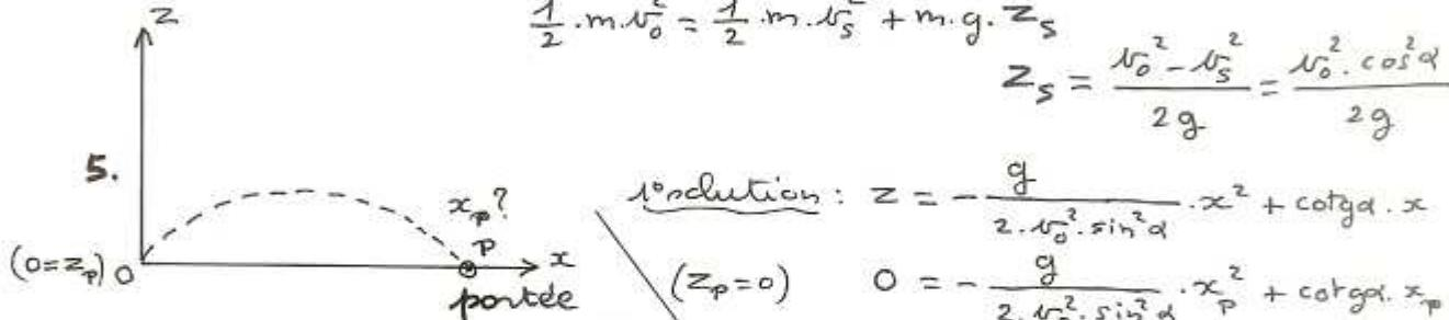
$$1^{\circ} \text{ solution: } z = -\frac{g}{2v_0^2 \cdot \sin^2 \alpha} \cdot x^2 + \cot \alpha \cdot x$$
