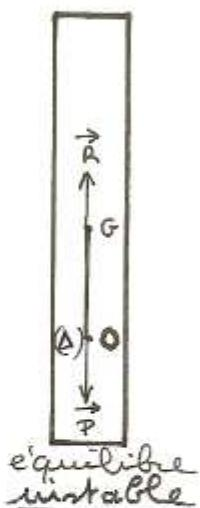
$$\begin{aligned} \sum \vec{F} &= \vec{0} \quad \vec{P} + \vec{R} = \vec{0} \\ \sum \alpha_f &= 0 \quad \alpha_f \vec{P}/D + \alpha_f \vec{R}/D = 0 \end{aligned}$$
