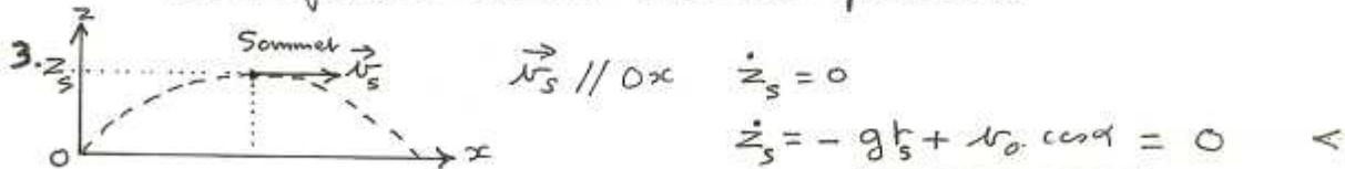
$$\vec{v}_s \left| \begin{array}{l} \dot{x}_s = v_0 \cdot \sin \alpha \\ \dot{z}_s = 0 \end{array} \right.$$
